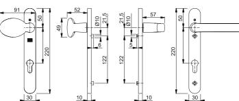
\* also available: 44mm door thickness Aluminium, brass and stainless steel door handles
